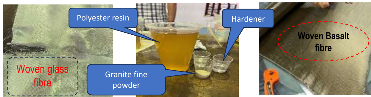
Figure 1. Material: matrix, resin, hardener, filler
