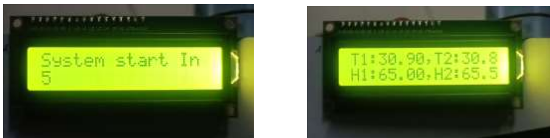
Figure 13. (a) LCD Display "System starts in 5" (left) and (b) LCD showing the surrounding temperature and humidity (right).
