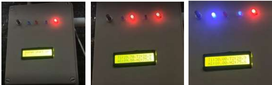
Figure 15. (a) LCD showing 'System start in 5' in Sinar Syukrawie Enterprise (left), (b) Temperature <30°C (centre), and (c) Temperature ≥30°C (right)
