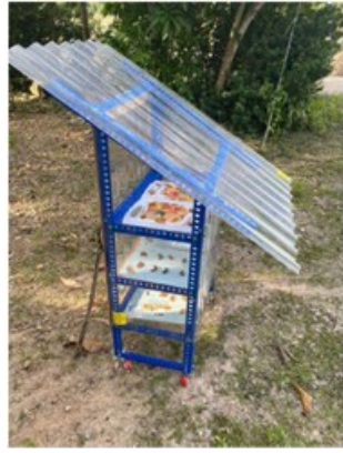
Figure 1. A construction of MOESUN, the mobile solar dehydrator
