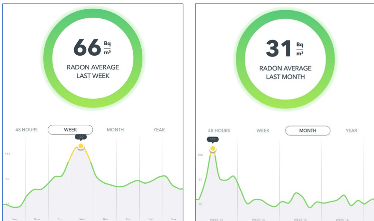
Figure 1. Radon monitoring inside storeroom at ground floor of two stories residential building.
