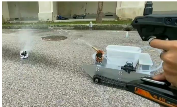
Figure 1: The Firefighter Robot with a Fire Suppression System
