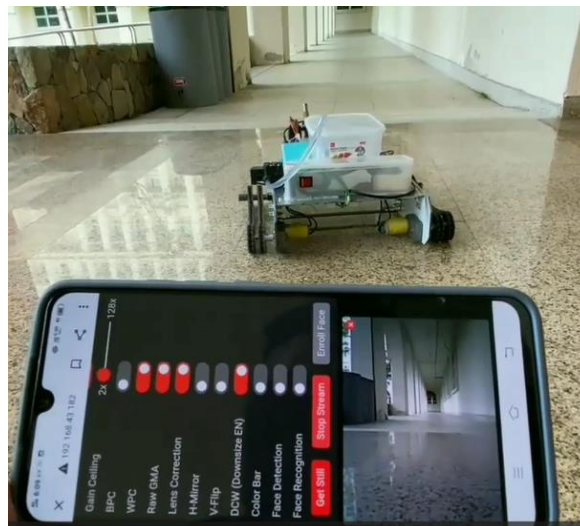
Figure 3: The Prototype of Firefighter Robot and Camera View from Smartphone
