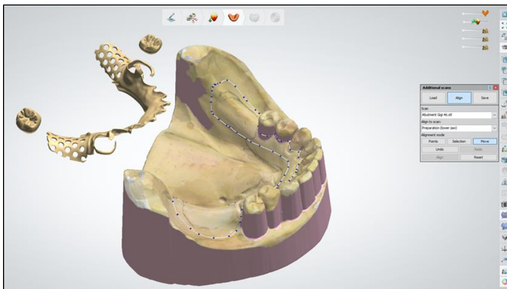
Figure 3.15 Integration of .stl Files of Abutment Teeth and Framework and Realignment Using Move Functions
