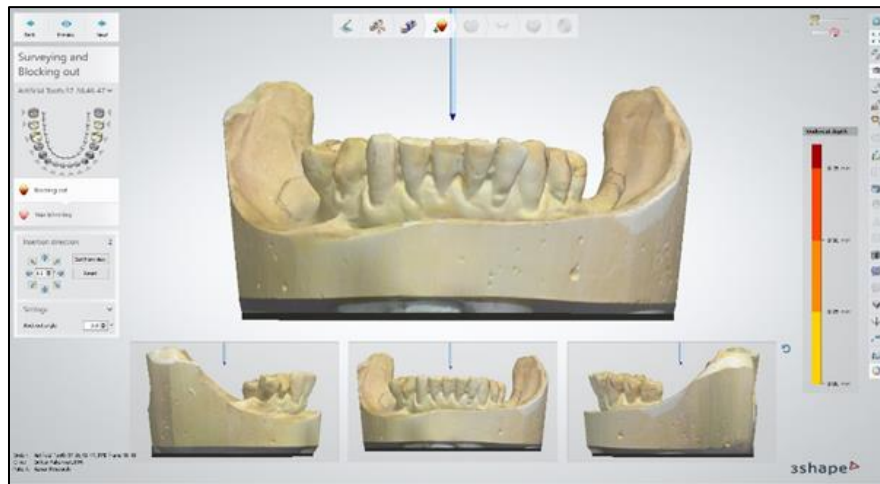
Figure 3.8 The Digital Surveying Process is Performed in the 3Shape Dental System
