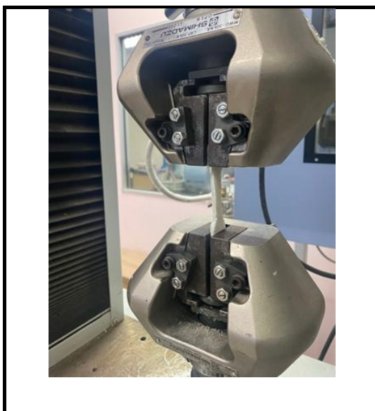
Plate 3.3 Example Depiction Of The Solid Propellant Sample Under Uniaxial Tensile Test
