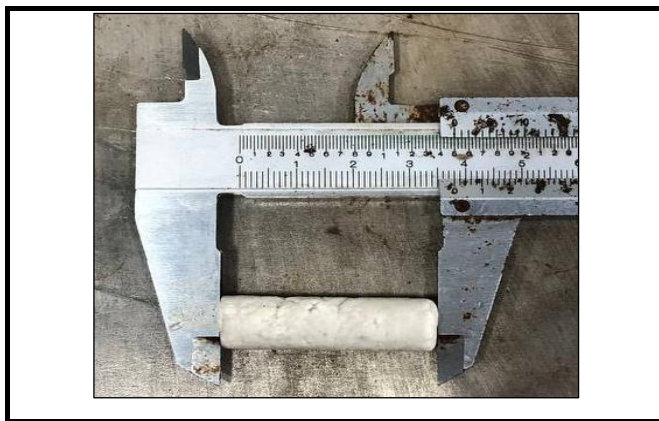
Plate 3.2 Measurement of Burn of Solid Propellant at Ambient Temperature and Pressure
