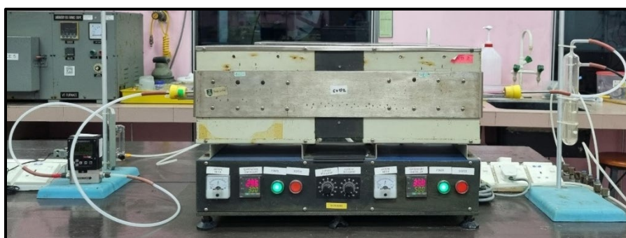
Figure 3.6 CVD with Double Furnace System
