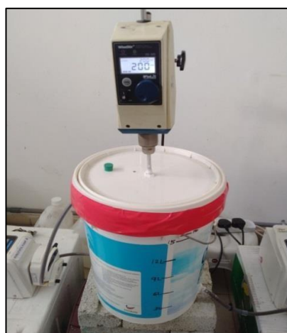
Plate 4.1 The Feeding Tank equipped with a stirrer
