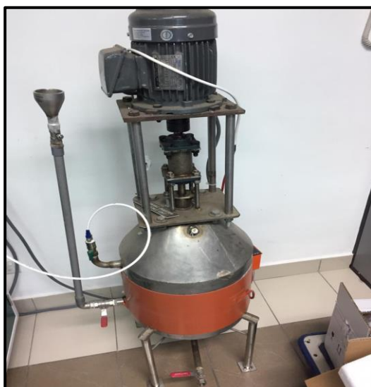
Plate 3.2 Picture of 40L digester (Pilot Scale)
