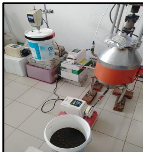
Plate 3.4 Set-up of the continuous feeding of IWK Sludge
