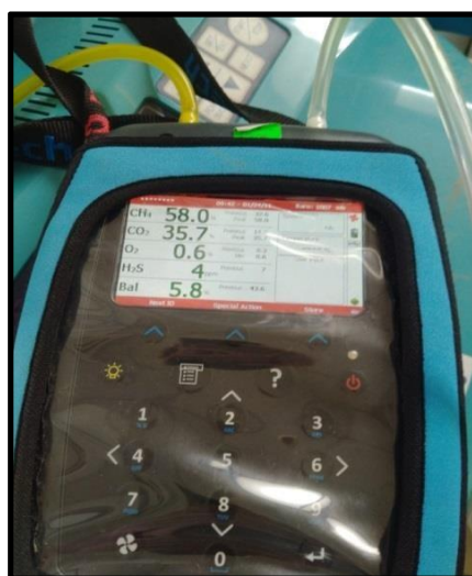
Plate 3.8 the portable gas analyzer features
