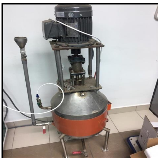
Plate 3.3 40L pilot digester of AcoD process at IWRC, KL
