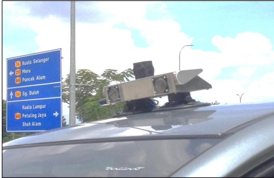
Figure 3.10 The 360° Camera View on RADIS 2.0
