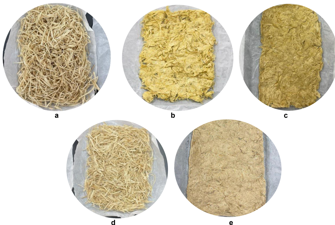
Figure 1: Image of nonwoven sheet samples; a – untreated, b – treated with 3% NaOH, c – treated with NaOH 5%, d – treated with H_2SO_4 7% and e - treated with H_2SO_4 10%.
