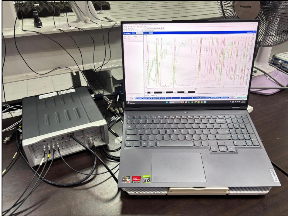
Plate 3.3 Simcenter Testlab Impact Testing Software and LMS SCADAS Data Acquisition
