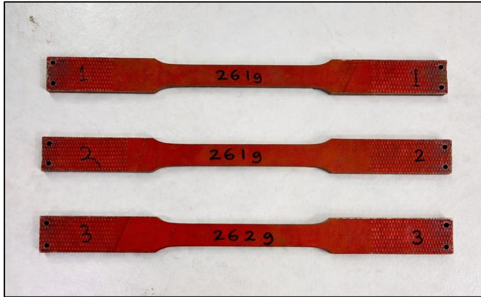
Plate 3.2 Steel Dog-Bone Specimens Used in This Study (Steel Specimen 1 to 3)
