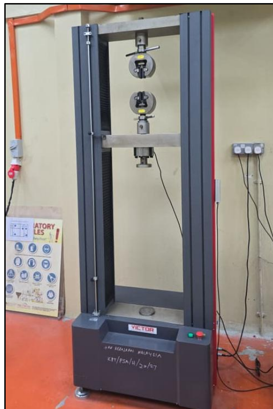
Plate 3.7 VEW2302A Universal Electromechanical Tensile Machine Used for Tensile Testing of the Steel Dog-Bone Specimen (60 kN Capacity)
