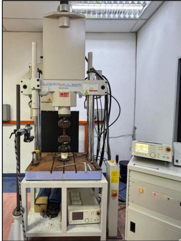
Plate 3.6 Shimadzu ServoPulser EHF-Series Servo-Hydraulic Universal Testing Machine Used for Tensile Testing of the Tobacco Composite Strip (10 kN Capacity)
