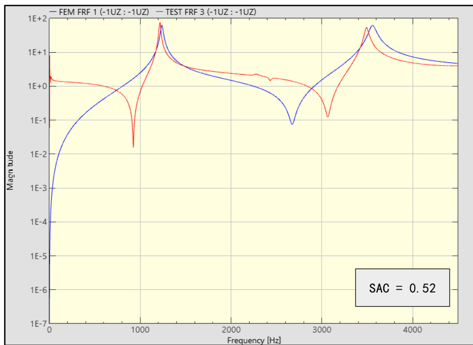
Figure 4.2 FRF Comparison Between EMA and the Initial FE Model for the Steel Dog-Bone Specimen for (a) Specimen 1, (b) Specimen 2, and (c) Specimen 3
