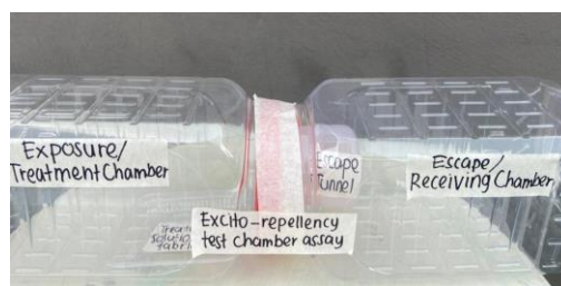
Figure 2: The 3D excitorepellency chamber assay from recycled materials used to assess the effects of extracted pomelo peel compared to a commercial insect repellent product
