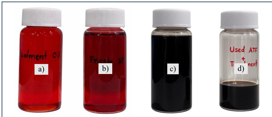
Figure 3.3 a) Treatment Oil, b) Fresh ATF A 0 , c) Used ATF A, d) Treated ATF A 1
