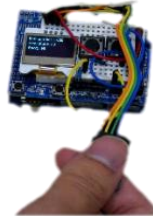
Figure 5: Completed OxyPulse prototype displaying live readings on OLED screen.
