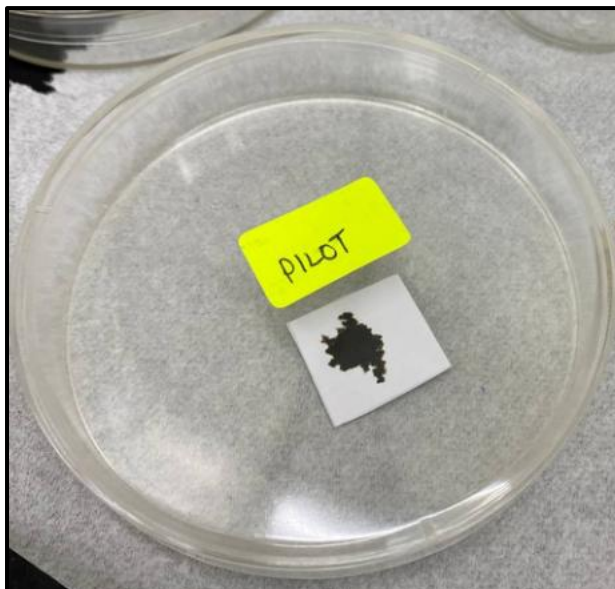
Figure 3.2 Prepared Ink-Stained Paper Section Measuring Approximately 1 cm \times 1 cm, Placed in a Clean Petri Dish and Labelled According to The Ink Brand.
