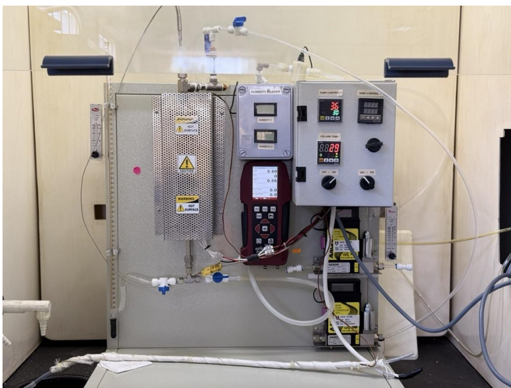
Figure 5.3 CO 2 Adsorption Pilot Plant
