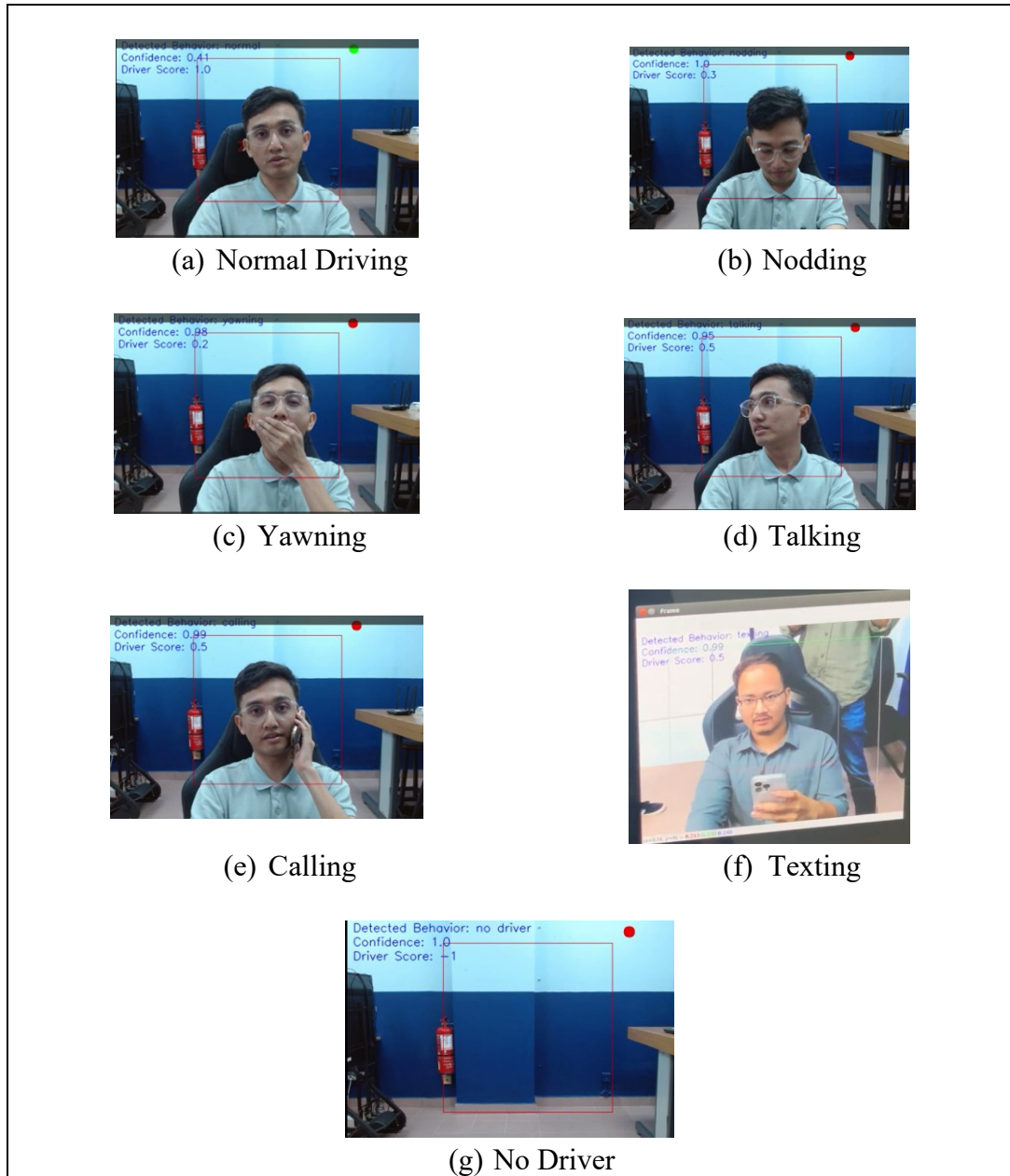
Figure 4.25 Real-Time Detection Results on Lenovo Ideapad Gaming 3 Showing Classification Outputs for Six Driving Behaviors: (a) Normal Driving, (b) Nodding, (c) Yawning, (d) Talking, (e) Calling, (f) Texting, and (g) No Driver.
