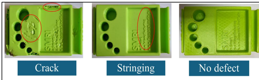
Figure 3.3 The Example of Defects on AM Products A) an Example of Crack Defect B) an Example of Stringing Defect C) an Example of No Defect.
