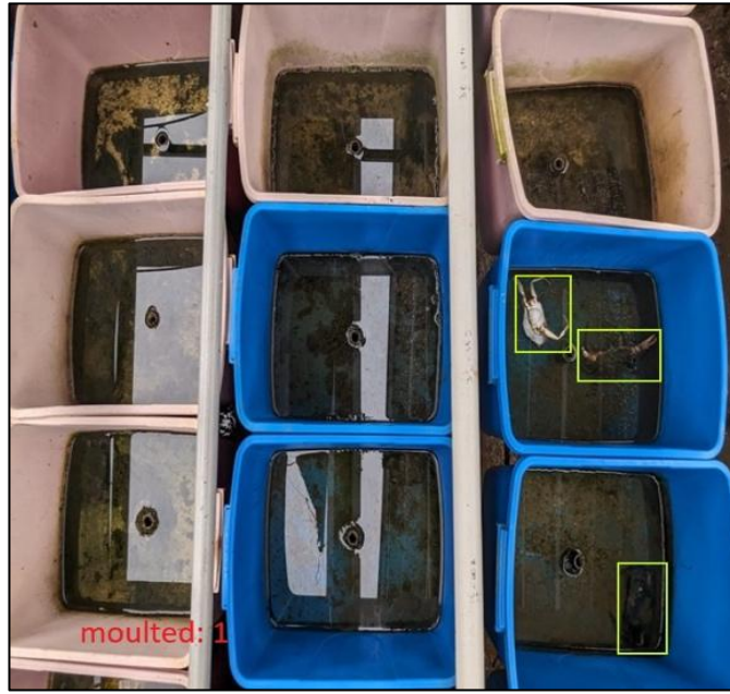
Figure 4.5 Moulted soft-shell crab detected with the IoT setup and YOLOv7 Object Detection
