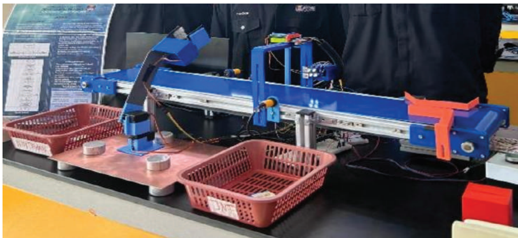
Figure 2. Robot Arms Attached Together with Conveyor System
