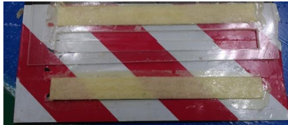
Figure 4: Compound hardened at surrounding temperature
