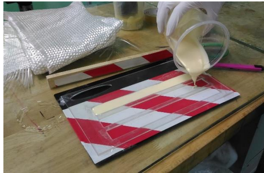
Figure 3: Pouring process of compound into cavity
