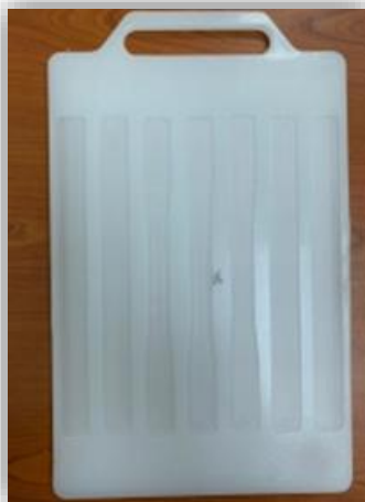
Figure 1: Single fibre mold made from plastic after machining by CNC
