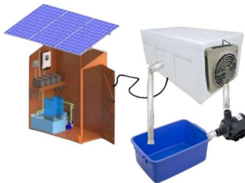
Figure 3: Prototype simple air Cooling / air conditioner
