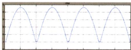
Fig. 15: Output voltage of R load
