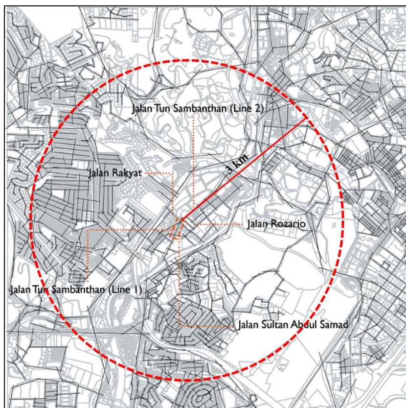
Figure 4. Axial map of the pedestrian and vehicle network for the 3 km radius from Little India, Brickfields. The axial map reveals the significant balance for both global and local integration value.
