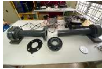
Figure 7. Impedence Tube Setup
