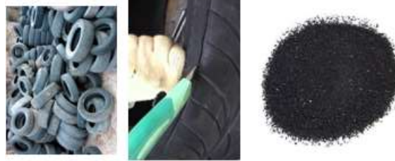
Figure 2. Rubber waste tyre preparation
