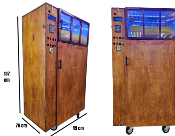
Fig. 2 Intelligent Seed Hub (ISH)- Innovative germination rack equipped with IOT system Source: Author (2026)
