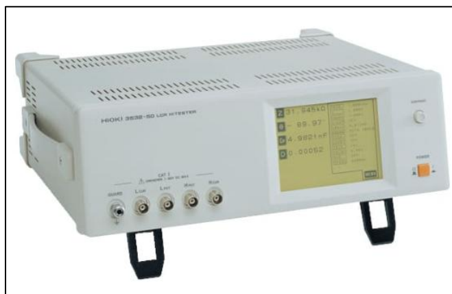
Figure 3.4 EIS instrument, HIOKI 3532-50 LCR Hi-TESTER PGZ100
