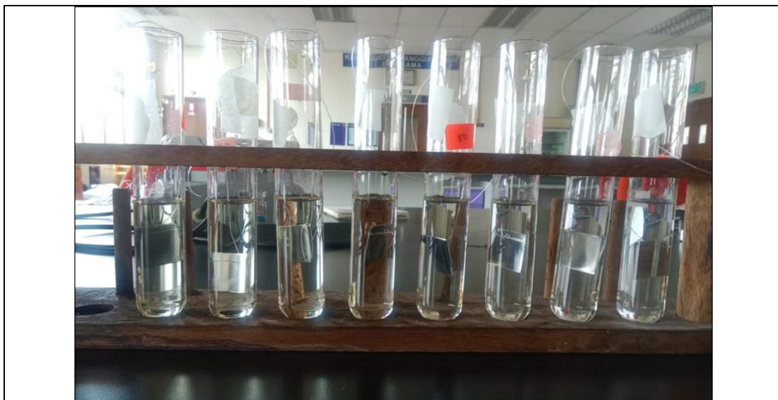
Figure 3.3 Immersion test or weight loss method
