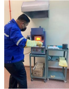
3. The sample was then placed in a ceramic crucible and melted the samples at 1050 °C in furnace
