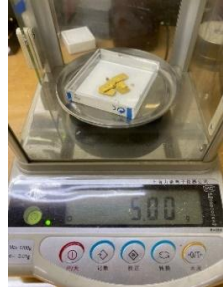
2. The combination of samples was weighed to give a total of approximately 5 grams
