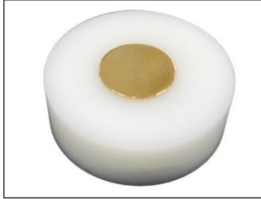
Figure 4.13 Gold Certified Reference Materials Known as MyREM Au in the Form of a Round Slice with a 12 mm Diameter Embedded in Plastic Discs with a 30 mm Diameter
