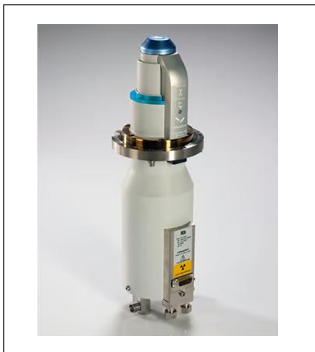
Figure 2.13 The EDXRF Tube Excitation Source Shines X-Rays from Below Up onto the Sample
