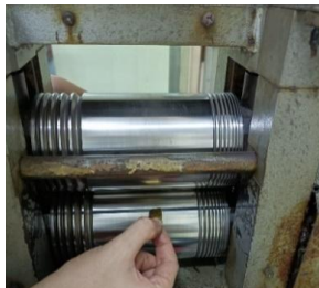
6. Rolled the sample to give 0.25-0.30 mm thickness
