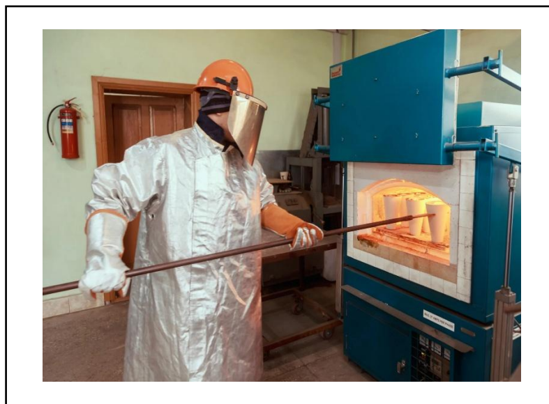
Figure 2.5 A process of cupellation in the furnace to melt the gold alloy samples
