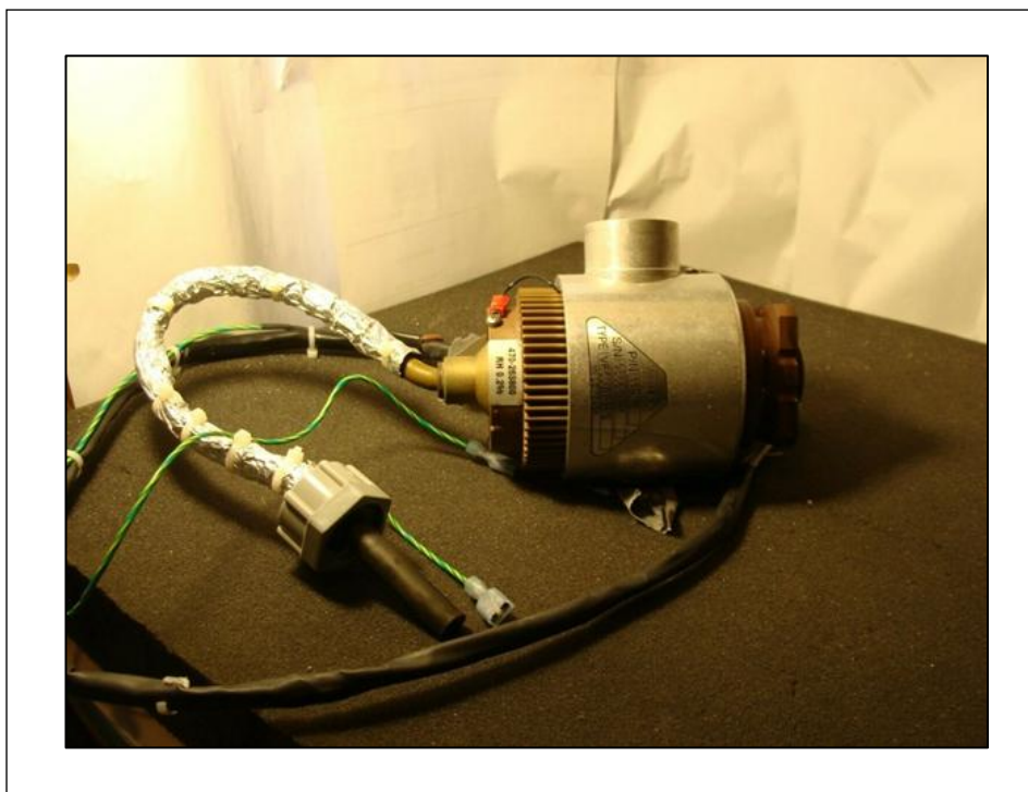
Figure 3.18 A High Flux 50 W Rhodium Anode X-ray Tube was used in this Study
