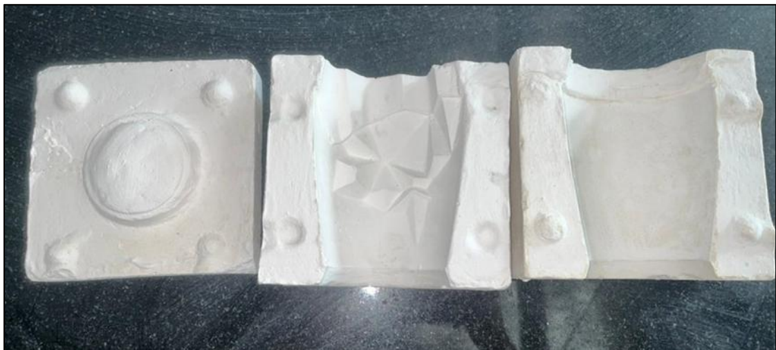
Figure 4.21 Surface Of RPOP 160°C + Silubit G80 (0.5%) Before Casting
