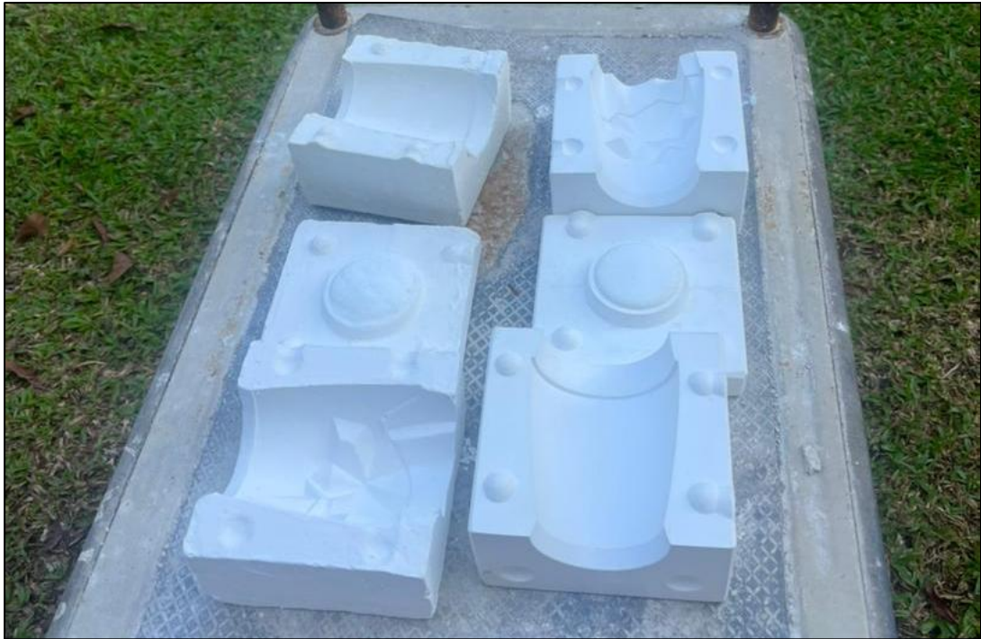
Figure 4.19 The Mould Drying Parts Of Mould On Air
