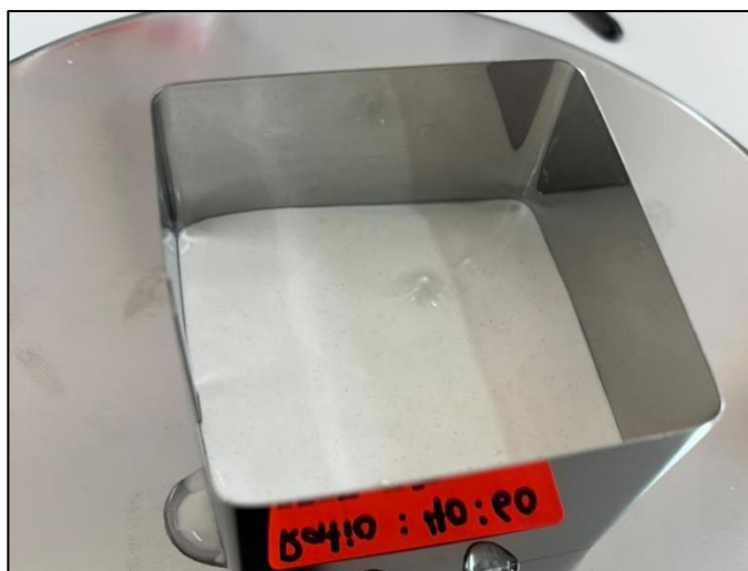
Figure 5.1 The RPOP In Room Temperature Does Not Harden
