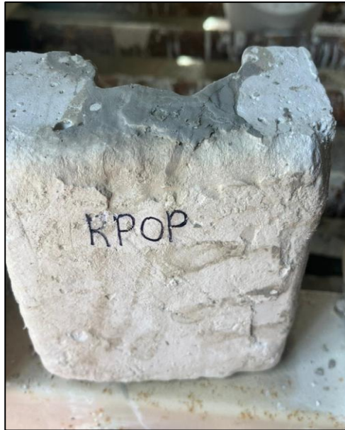
Figure 4.23 Mould RPOP + Silubit G80 Which Has Been Damaged After Casting
