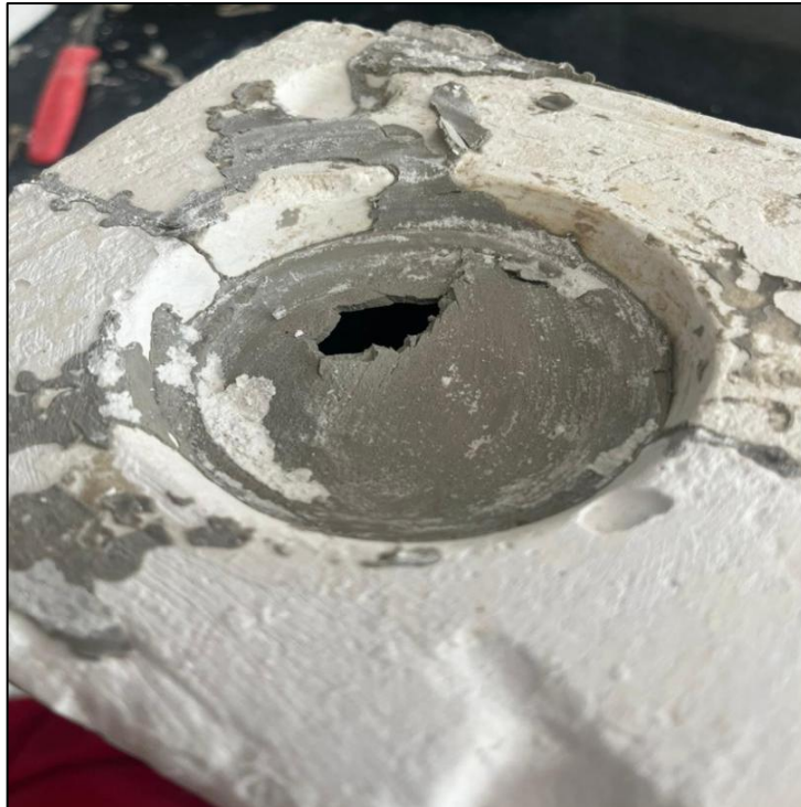
Figure 4.25 Slip Cast Part Torn Due To Sticking To The Mould
