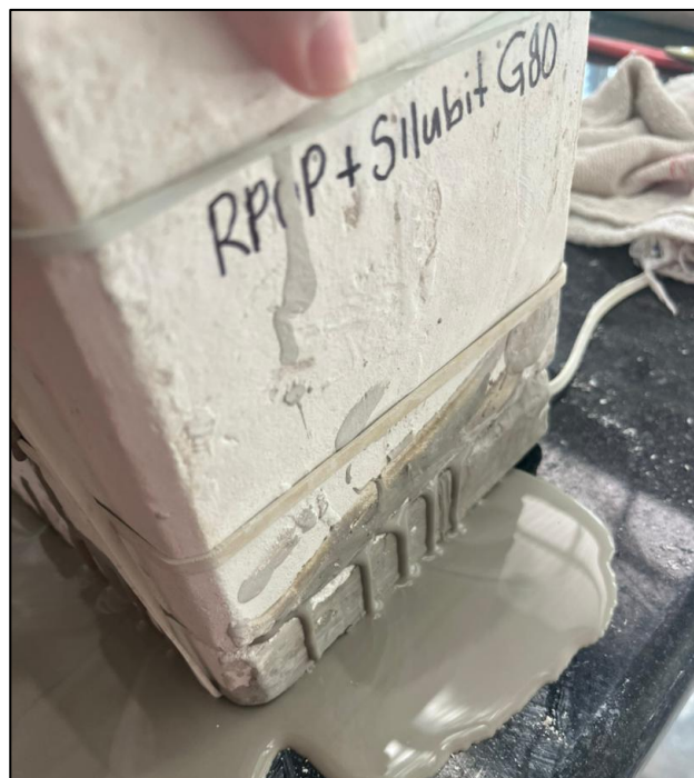
Figure 4.24 Mould RPOP + Silubit G80 Damaged Causes Slippage To Occur
