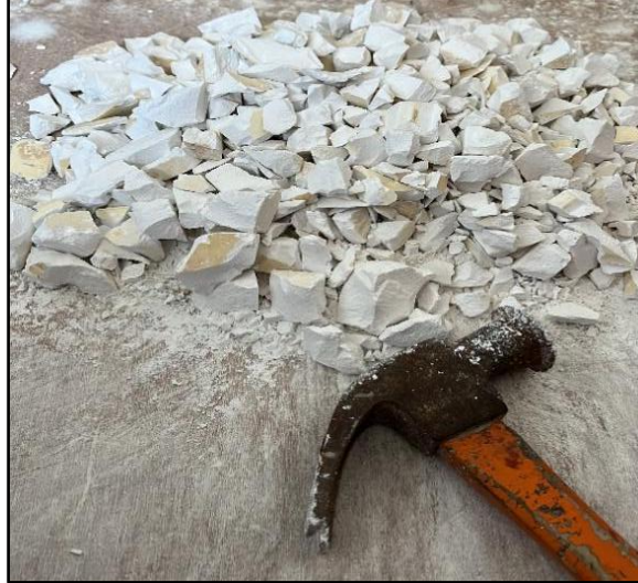
Figure 3.2 Break Used Mould Into Small Pieces.
