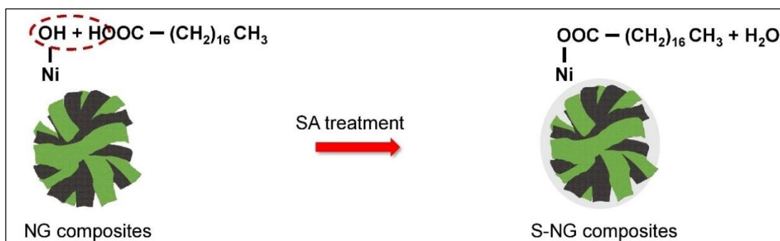
Figure 4.6 Chemical Reaction during the SA Treatment Process to produce Optimally Hydrophilic S-NG Composites Powder
