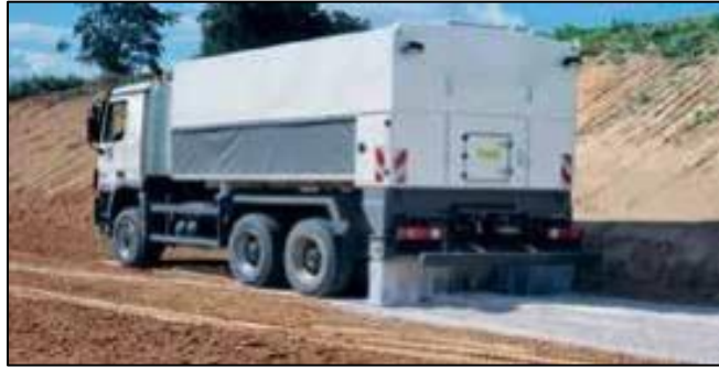
Figure 3-10 Desirable Features of a Mechanical Spreader Include Load Cells, Apron, Variable Width Spreading, Sealed Tanker and Filters for Binder Intake Management. (Source: Stabilised Pavements (M) Sdn. Bhd.)
