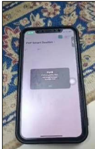
Figure 4. The Blynk app alert via the smartphone, triggered by full bin detection
