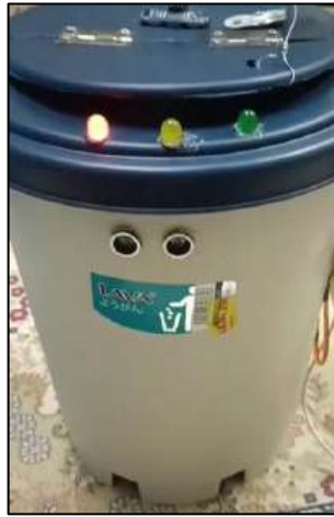
Figure 3. Hardware prototype in operation showing red LED activation on the smart dustbin, triggered by full bin detection
