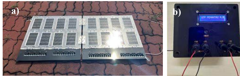
Figure 1. a) Customised flipped bookcase solar panels with b) PV monitoring system
