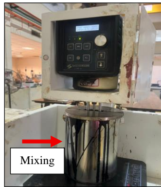
Fig. 3. The blending and mixing process by using the Silverson machine at the required speed and time.
