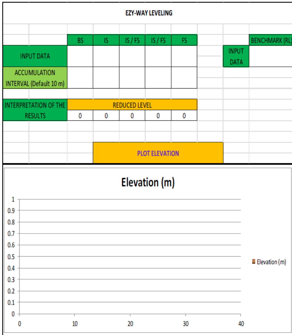
Figure 2: The proposed EZY-WAY Leveling tool.
