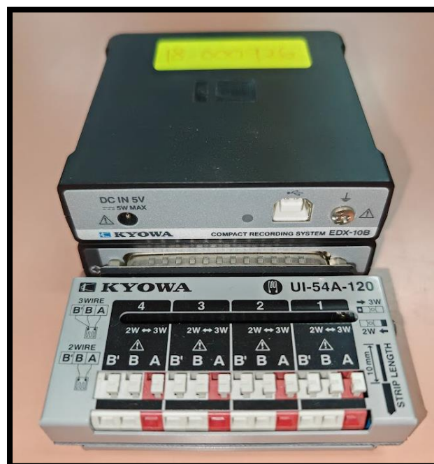
Plate 3.7 Kyowa Strain Measurement and Data Acquisition System
