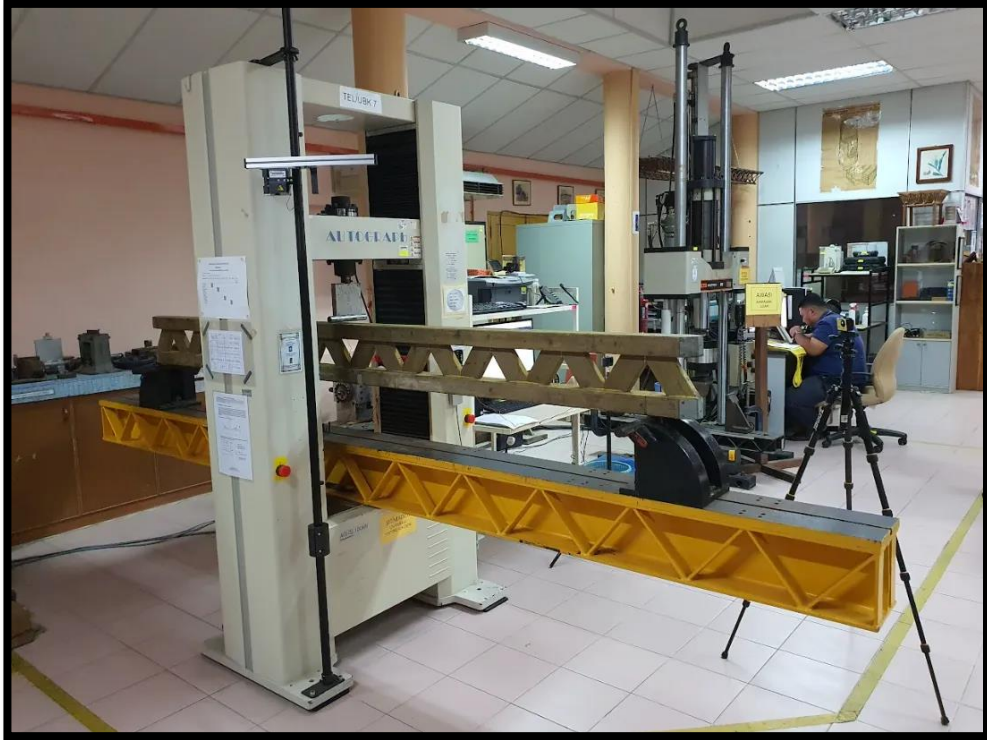
Plate 3.10 Specimen ETN131 Prepared for Flexural Bending Test.
