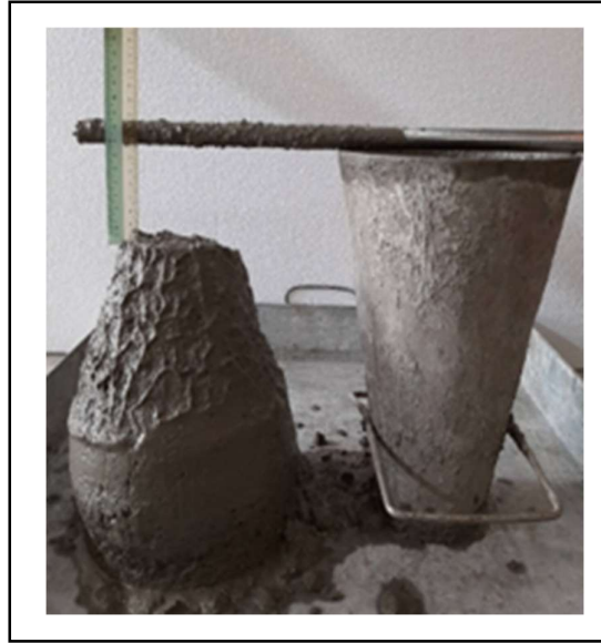
Figure 3.15 Slump Measurement of Fresh Concrete
