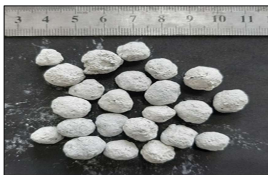
Figure 3.5 Green Artificial Aggregate (GAA) of 10 mm Size Used for Replacing NA
