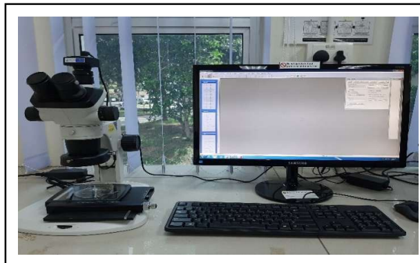
Figure 3.33 The Workstation for Stereo Microscope Used for Observing Morphological Structure of Aggregates and Water Movement from Aggregates to Cement Paste
