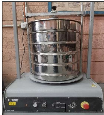
Figure 3.6 Sieve Shaker Used to Determine the Particle Size Distribution of Aggregates
