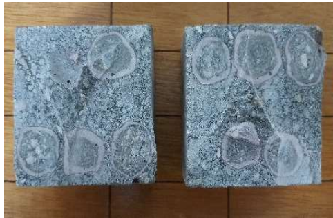
Figure 3.32 The Procedures for Colour Propagation Test Using Stereo Microscope
