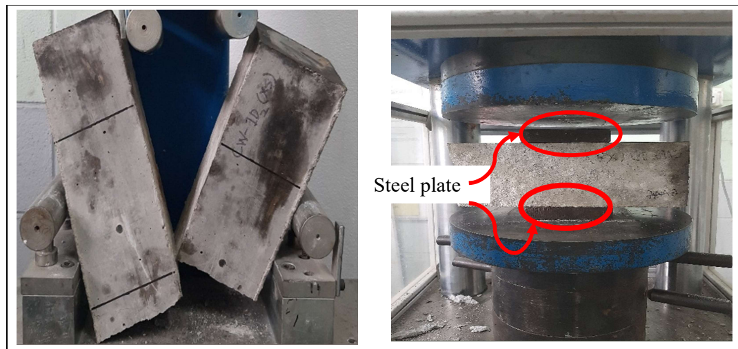
Figure 3.21 The Broken Prism Specimens and the Set Up For Modified Compression Test
