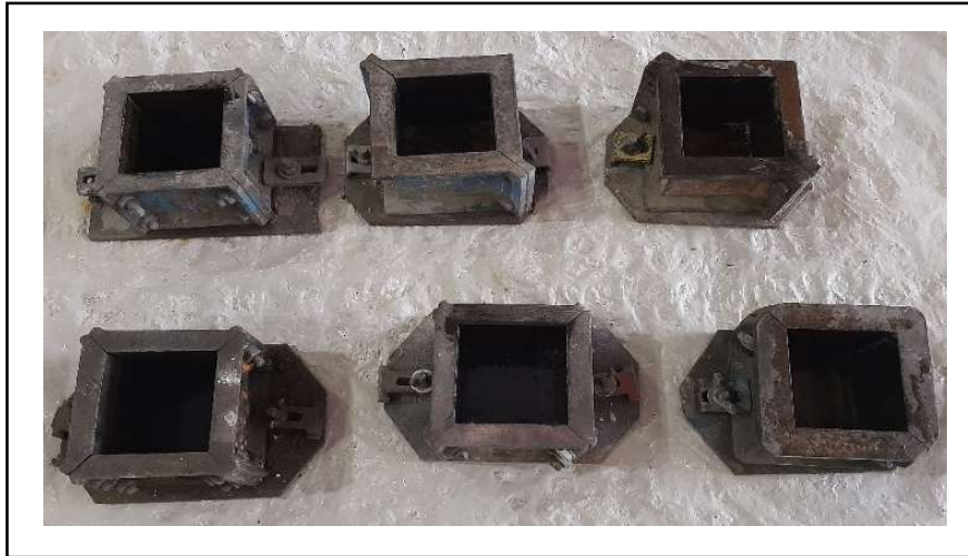
Figure 3.11 Steel Moulds that Ready for Casting
