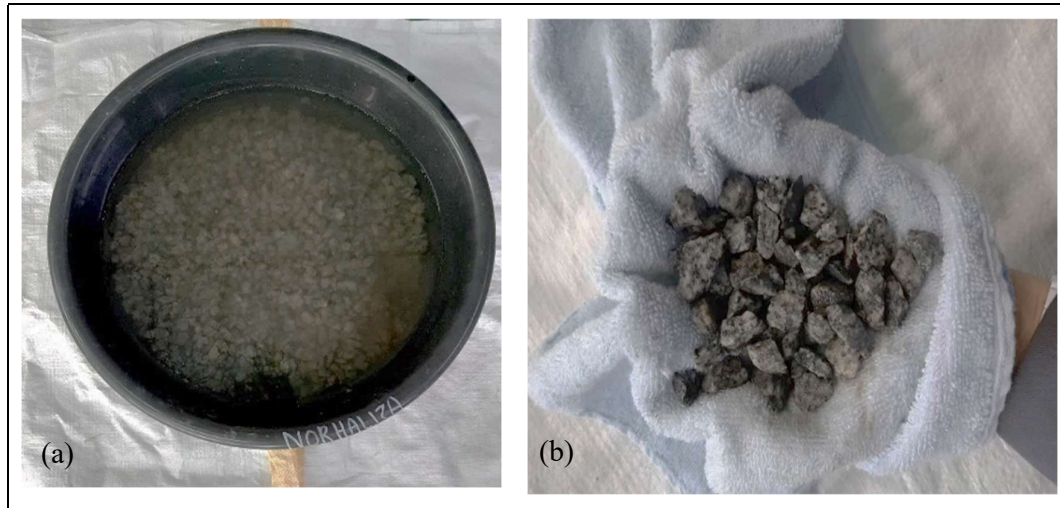
Figure 3.14 Process to Produce SSD Condition of Coarse Aggregates (a) Immerse the Aggregate in the Water for 24 hours and (b) Rolling up the Aggregate into the Towel
