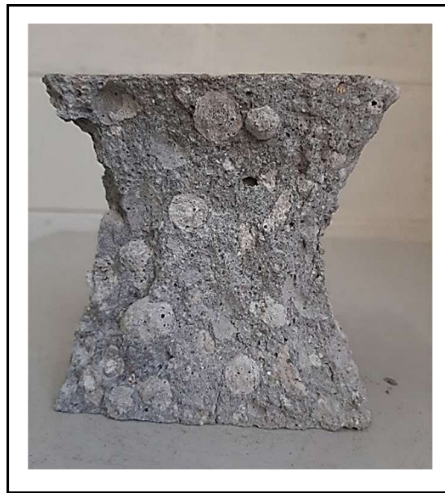
Figure 3.24 Failure Pattern of Cube Concrete
