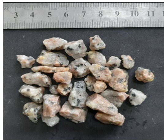
Figure 3.4 Natural Aggregate (NA) of 10 mm Size Crushed Granite
