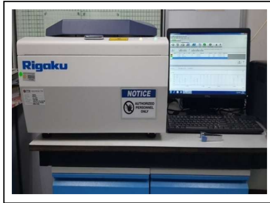
Figure 3.28 XRF Equipment Used to Determine the Chemical Composition of Cement and GAA
