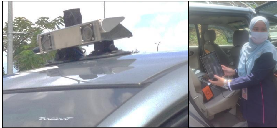
Figure 3.9 The RADIS Tool Attached to the Survey Vehicle
