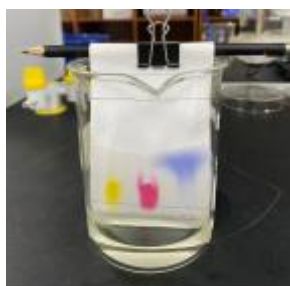
Figure 4.3 Developer solution (isopropyl) should be poured into the beaker and let rise.
