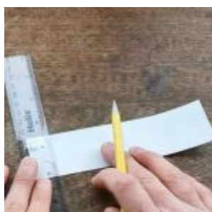
Figure 4.1 Take a strip of chromatography paper and make a line around 1-2cm.
