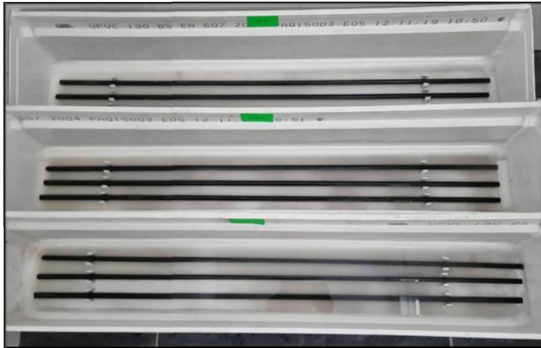
Figure 3.48 The Treatment Of Reinforcing Bars In Inhibitor Solution
