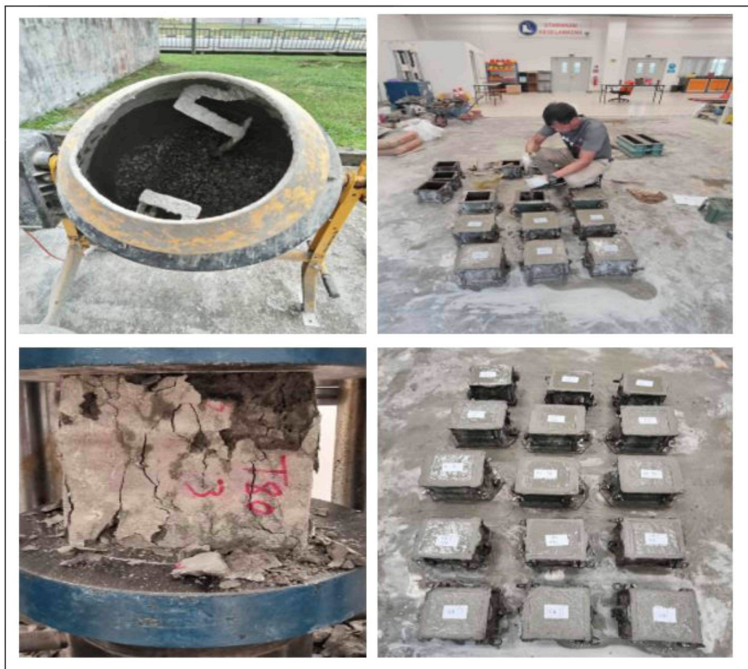
Figure A.10 Sample Preparation for the f_c Test
