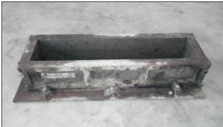
Figure 3.43 The Beam Mould (500 mm × 100 mm × 100 mm) Used For Specimen Preparation
