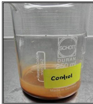
Figure 4.26 The 0.9% NaCl (Negative Control) Solution After Immersion Of Mild Steel Bars Coupons For 100 Days
