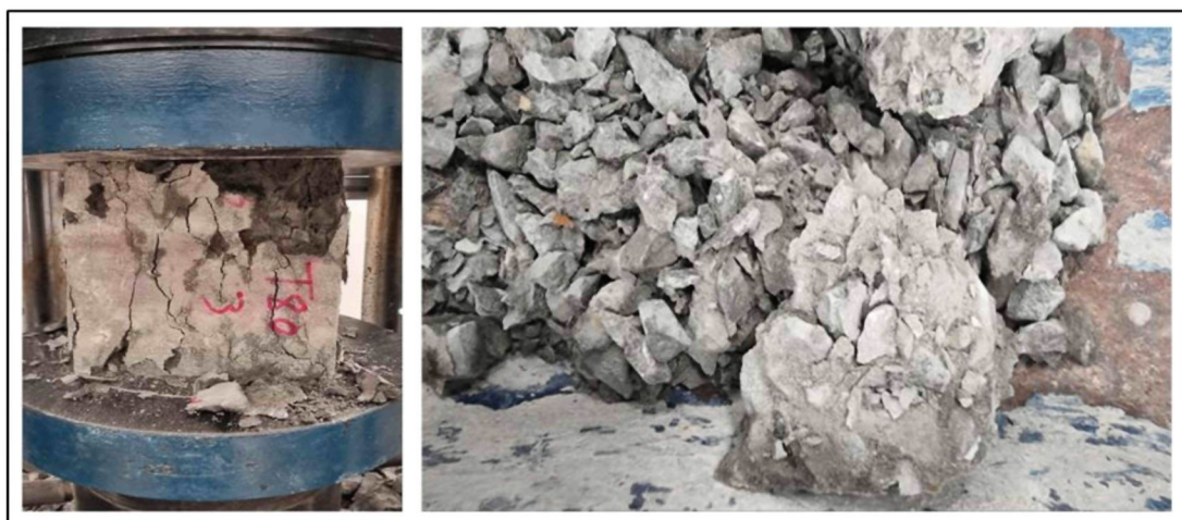
Figure 4.46 Explosive Failure Of Concrete Cubes Specimens Containing 10% Tween 80 Due To Brittle Behaviour
