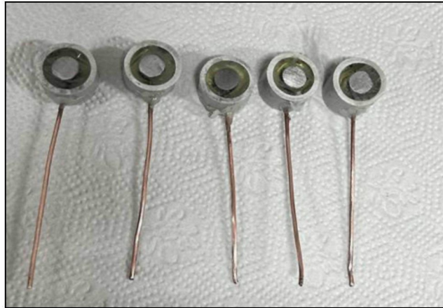
Figure 3.27 The Soldered Mild Steel Before EIS Analysis
