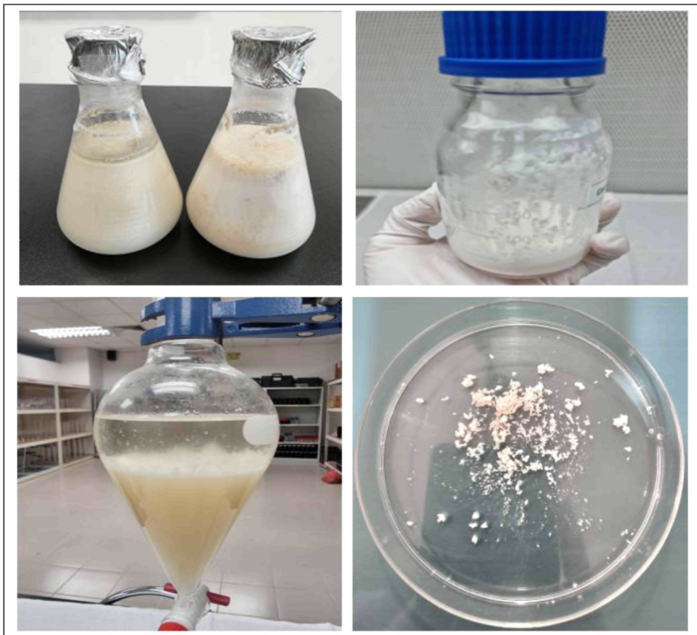
Figure A.2 Separation Process of Crude Biosurfactant from Liquid to Crystalline State
