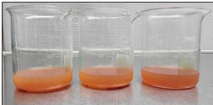
Figure 4.27 The Tween 80 Solutions After Immersion Of Mild Steel Bars Coupons For 100 Days (Positive Control)
