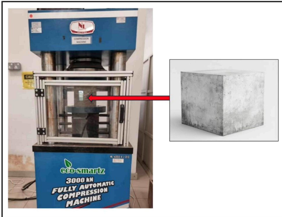
Figure 3.41 The Measurement Setup Of The Concrete Cube f_c
