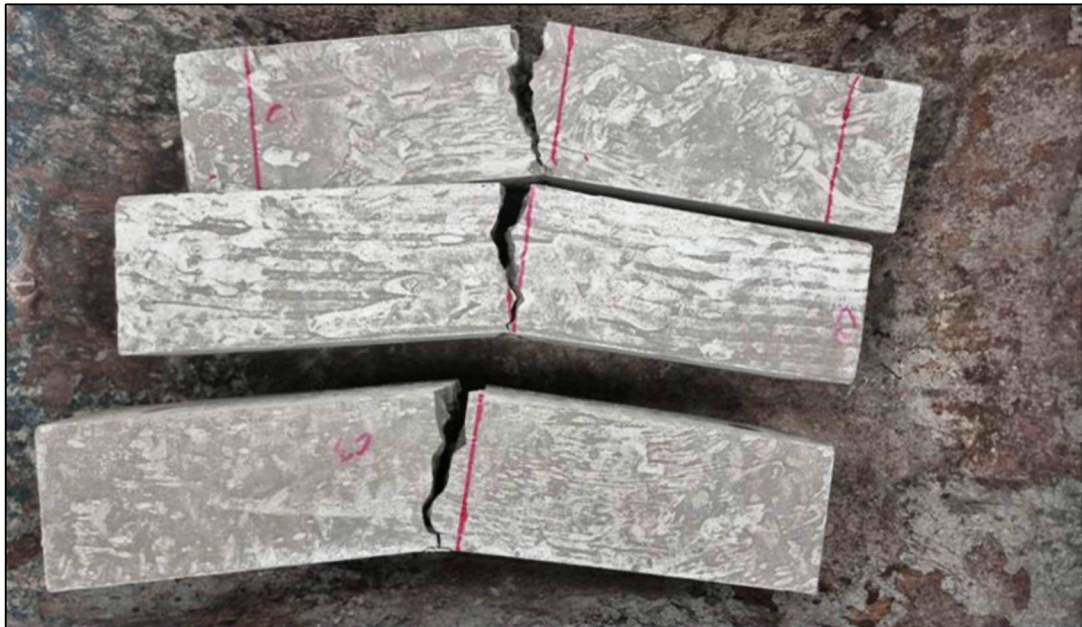
Figure 4.50 Biosurfactant Flexural Failure Pattern Of Singly Reinforced Concrete Beams With 10% Biosurfactant.
