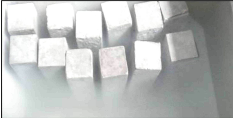
Figure 3.45 The Specimens in the Curing Tank At 25 \pm 2^\circ\text{C} For 28 Days
