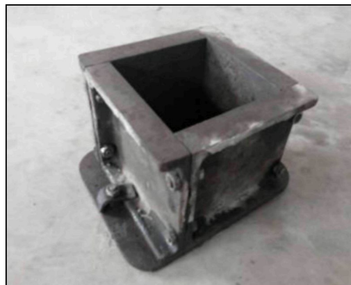
Figure 3.39 The 150 mm × 150 mm × 150 mm Cube Mould Used In This Study
