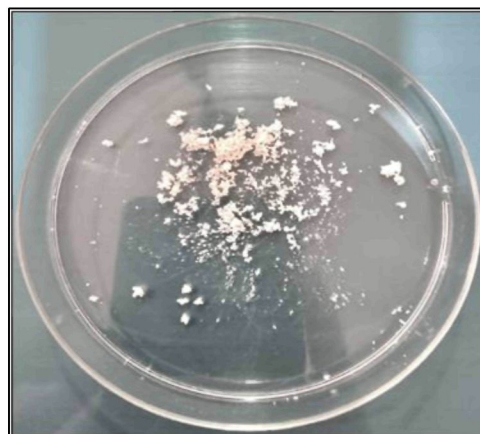
Figure 3.16 The Crystallized Biosurfactant After Evaporation
