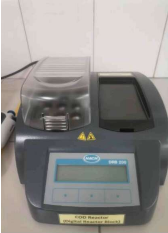
COD Reactor (Digital Reactor Block)
