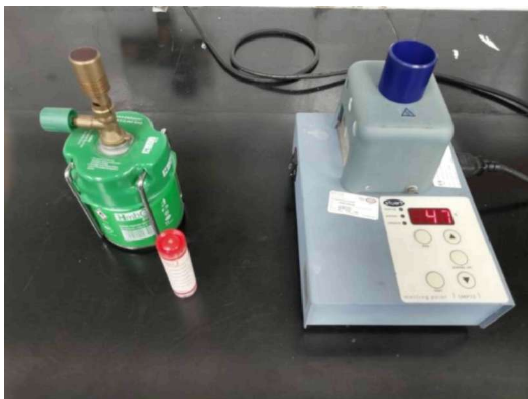
Figure A. 2d. Digital Melting Point with Capillary Tube Red Tip G0553
