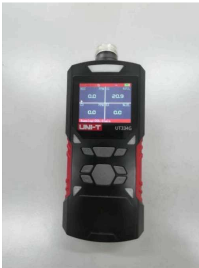
Figure A. 2s. Multi Gas Detector Leakage
