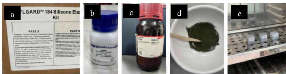
Figure 3.1 a) Poly dimethylsiloxane Kit, b) Pure Tin Powder, c) Copper Tin Alloy, d) Mixture of Metal and Polymer and e) Heating Process in Oven at 100 \text{ }^{\circ}\text{C}
