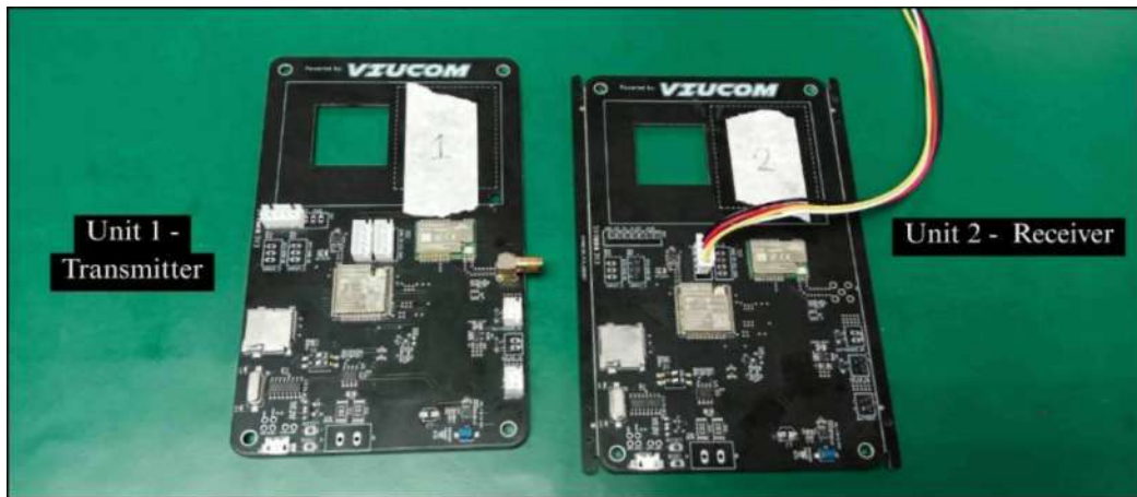
Figure 4.7 Finalized PCB Layout for GST Module (Unit 1 and Unit 2)
