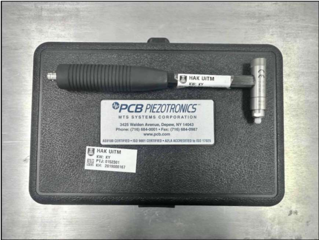
Plate 3.2 Impact Hammer Used in Testing
