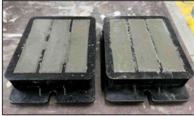
Plate 3.15 Three (3) Specimens of 160 x 40 x 40 mm Bar for Each Different Percentages
