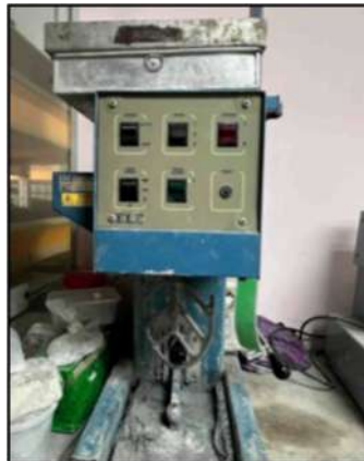
Plate 3.13 Mixer Used for Preparation of Mortar Cubes
