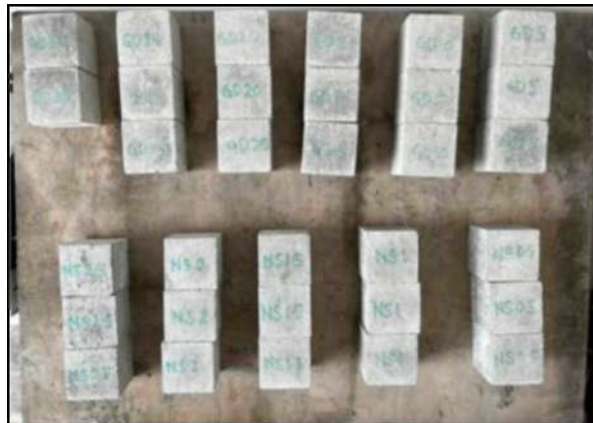
Plate 3.22 Specimens of 50 mm Cubes for Each Different Percentages for Compression Test
