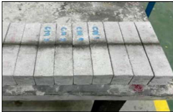
Plate 3.18 Patched Fracture Damage of Specimens on Different Type of Mortar Bars
