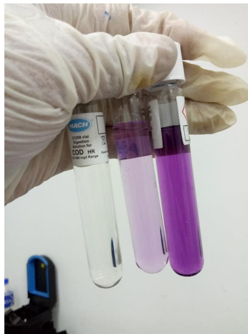
Figure 5: The right tubes is the water samples treated with millscals, in the middle tube was treated using magnetite.
