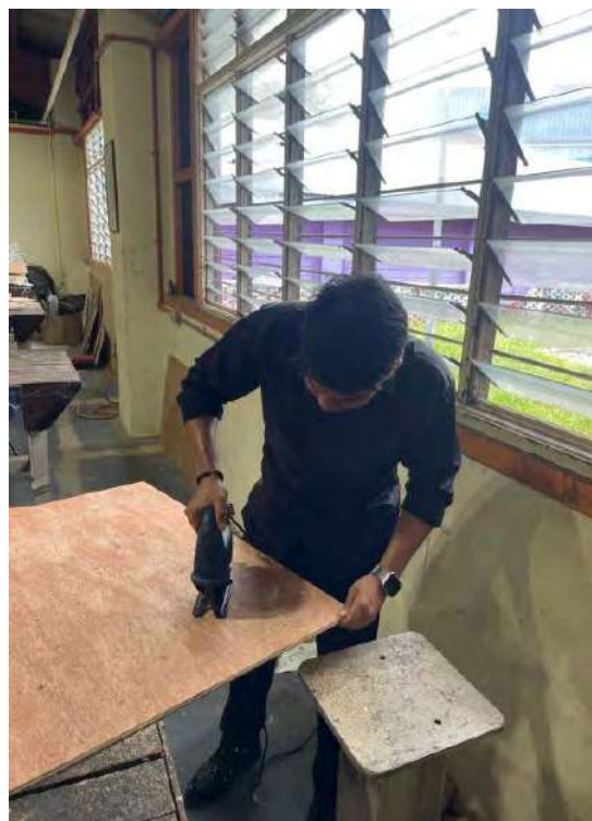
Figure 1.2 Cut plywood boards into circular shapes using a jigsaw.
