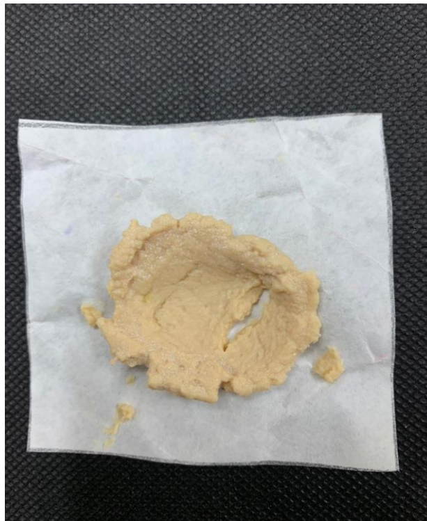
Figure 5: Plastic (dried casein) prepared at 60 °C using 10 ml of 0.1 mol dm -3 acetic acid
